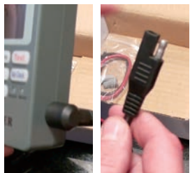
Connect timer and wiring harness using the "elbow" DIN connector (LEFT), then connect timer to motor using the "trailer" connector (RIGHT).
