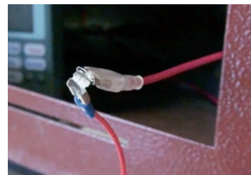
Connect timer (female) to solar panel (male) as shown in the photos above. Once mated, slide each connected pair onto the positive and negative terminals of a 12V battery (not included). Be certain to connect red-to-red (positive) and black-to-black (negative). Failure to do so can damage your solar panel.
