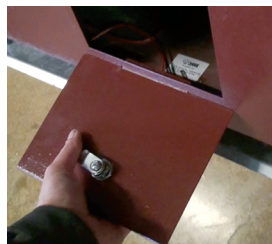
Open accessory door to locate timer and access all wiring
